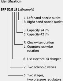
BFP 52E sizes 3 and 5 oil pumps are designed for small/medium-sized 2-stage domestic oil burners up to 42 l/h.
