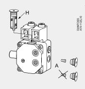
2-pipe operation: screw fitted
